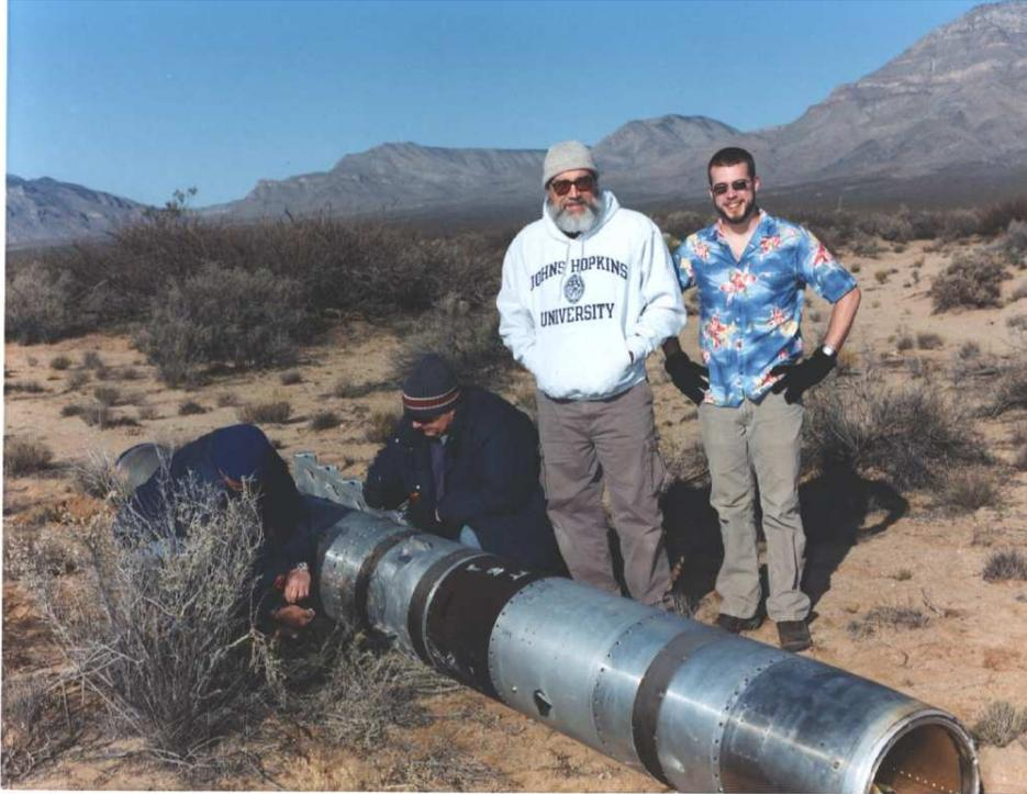
Figure A.19 Recovery operations for 36.198 at White Sands Missile Range, 2001 February 10. JHU engineer Russ Pelton and the author are shown. The payload is then transported back to the VAB for disassembly and shipping.
