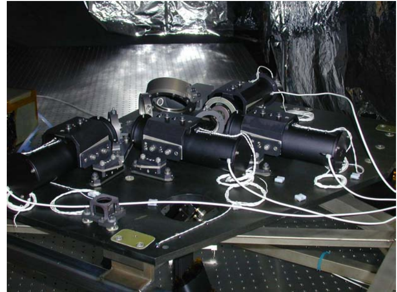
Calibration platform in CU vacuum calibration chamber. All optical components mounted in final locations except for lamps, which are being adjusted in translation. nominal positions.
