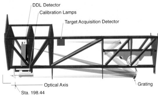
Figure 1. Schematic of the COS primary FUV channel (as proposed). Light is received from the HST OTA through an aperture (lower left), is dispersed by a concave diffraction grating, and finally is recorded on a curved double delay-line MCP detector adapted from the FUSE mission. The target acquisition detector has been replaced in current designs. The secondary NUV channel is fed by a fourth optic on the grating select mechanism.
