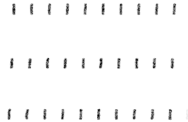
Figure 4: A portion of a slit image taken using the COS flight detector. The slits are 25 \times 500 \mu\text{m} on 200 \mu\text{m} centers. Each row is separated by 2.5 mm.
