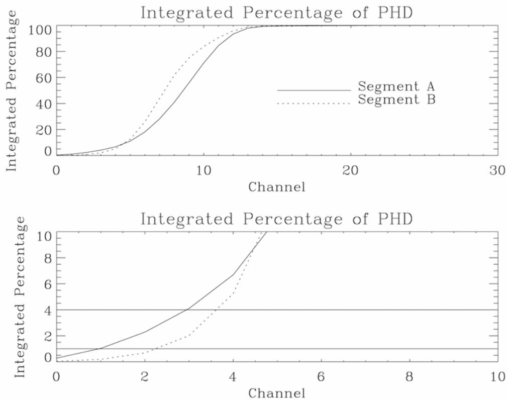
Figure 5.3-3: The integrated pulse-height distribution for FUV01 segments A and B. The top panel is full scale and the lower panel shows the same data, but with an expanded y-scale. The horizontal lines in the lower panel represent 1% and 4% loss of detection quantum efficiency. The vertical line denotes the maximum allowable change in the modal gain before the spectra must be repositioned on the detector.
