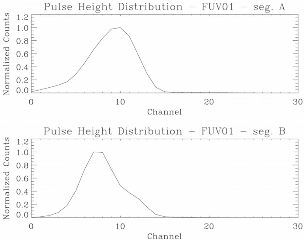
Figure 5.3-2: This figure presents the pulse-height distribution from FUV01 segments A and B in 5-bit resolution mode, the digitization used in TTAG mode.
