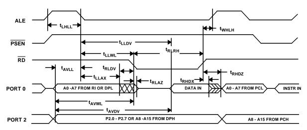
Figure 7. External Data Memory Read Cycle Waveforms
