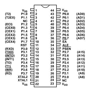
Figure 2b. UT69RH051 44-Pin Flatpack Connections
