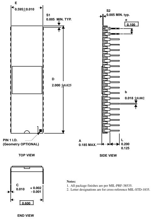
Figure 11. 40-pin Side-Brazed DIP
