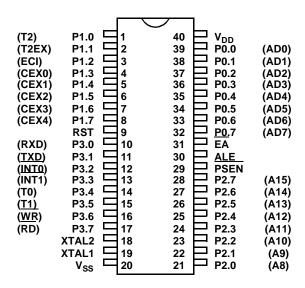
Figure 2a. UT69RH051 40-Pin DIP Connections
