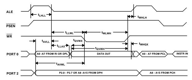
Figure 8. External Data Memory Write Cycle Waveforms
