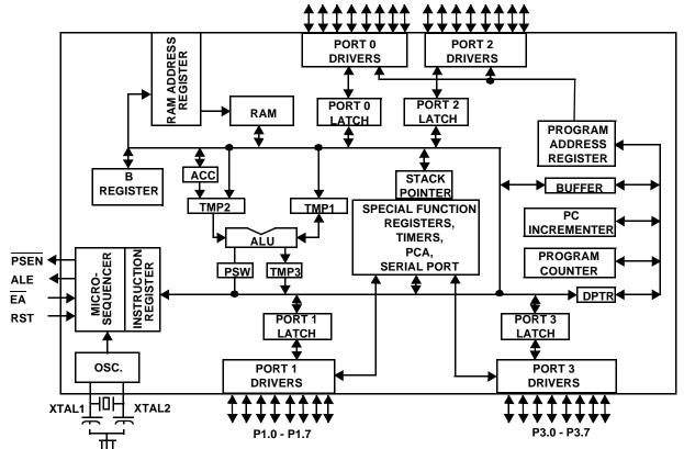
Figure 1. UT69RH051 MicroController Block Diagram
