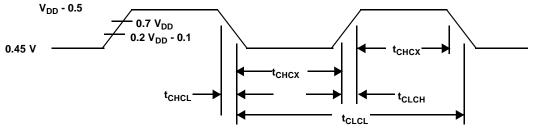
Figure 10. External Clock Drive Timing Waveforms
