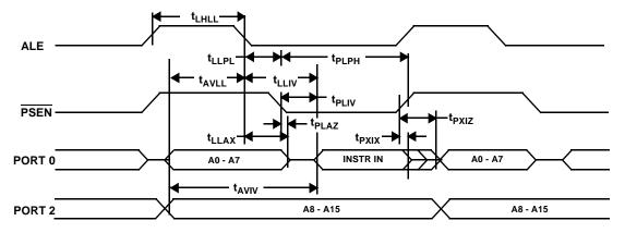
Figure 6. External Program Memory Read Timing Waveforms
