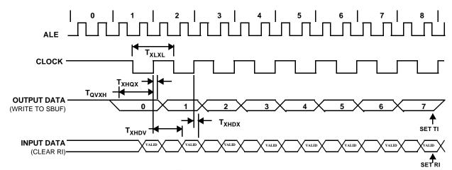
Figure 9. Serial Port Timing Waveforms
