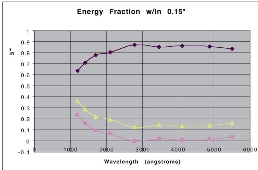
Figure 3.3 : The wavelength dependent filling factor for a 0.15 arc-second resolution element. The blue (top) line is the encircled energy within a 0.15" LSF. The yellow line represents the calculated filling factor ( $1 - EE$  for the LSF). The red line is the yellow line adjusted so that at 2780Å the filling factor is zero. The red line represents the wavelength dependent scatter contribution to the filling factor.
