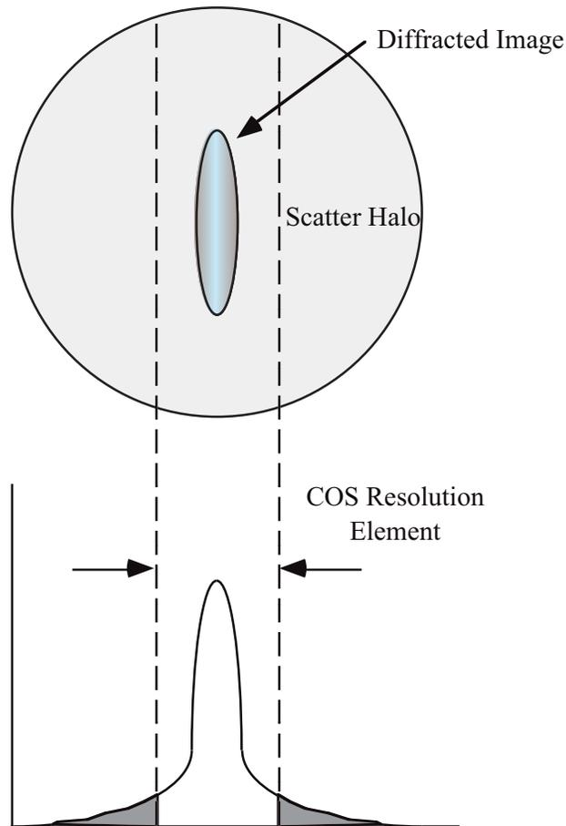
Figure 3.2 : The upper portion represents the aberration-corrected image with a circular scatter halo. The lower panel shows those portions of the LSF, which were integrated to form the filling factor.
