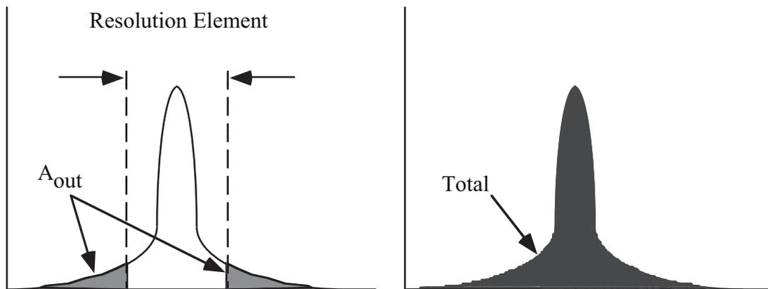
Figure 3.1 : The figure on the left shows where the LSF is integrated to calculate the filling factor of delta function absorption line. The right hand figure shows the total area under the LSF. The filling factor is then  $A_{out}/Total$ .
