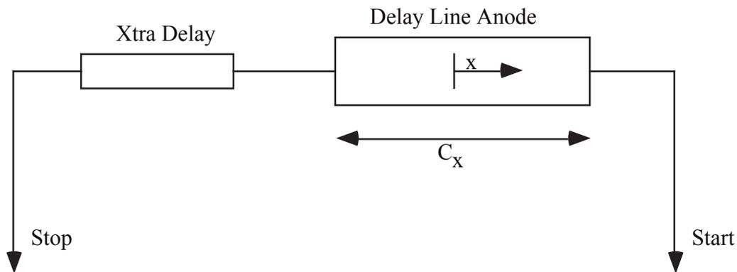
Figure 1: Schematic representation of the time delay concept. The Xtra delay ensures that the Stop signal always arrives after the Start signal.  $C_x$  is the physical length of the delay anode;  $x$  is the position of the detected photon.
