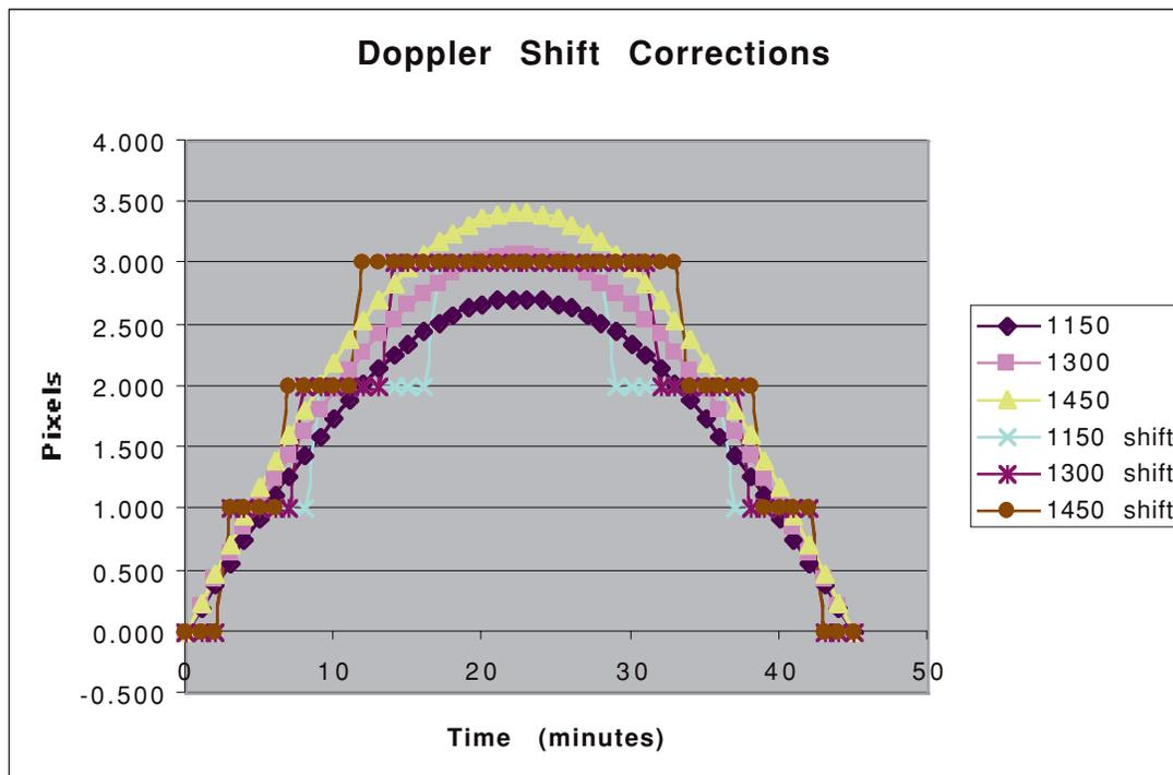
Figure 2: This figure depicts the continuous Doppler shift and the pixelated Doppler shift correction that will be used while in ACCUM mode to compensate for the spacecraft induced Doppler shift. Note how there is often a +/- 1 pixel error in the Doppler shift due to differences in the wavelength dependent Doppler shift.
