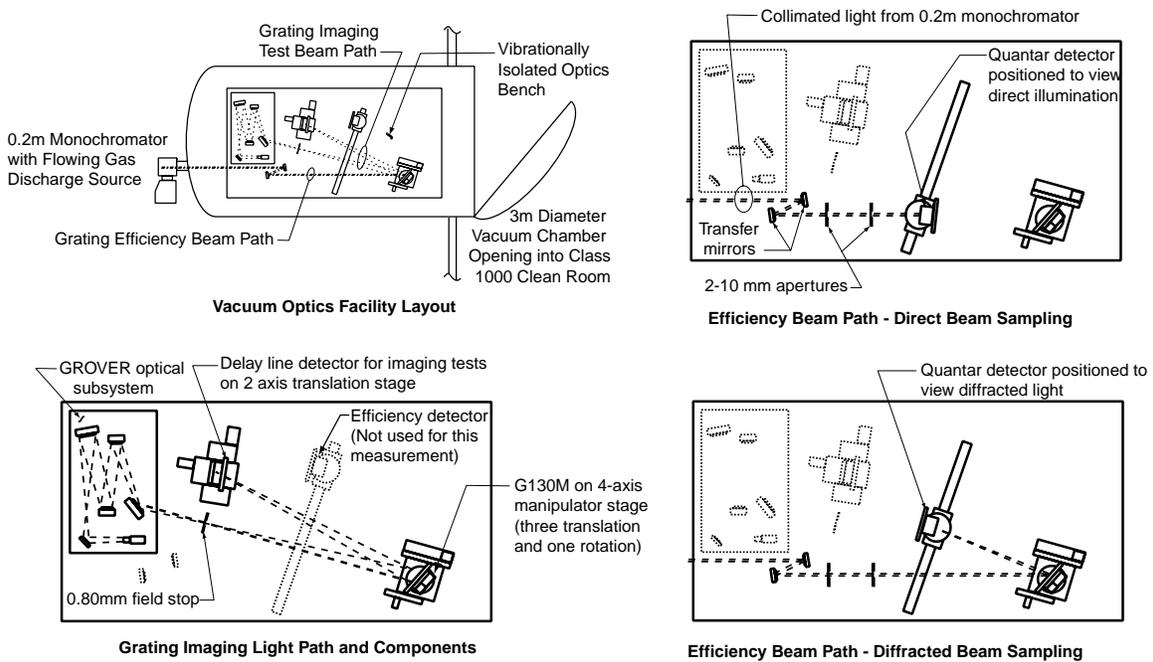
Figure 1: Grating resolution and efficiency test setups
