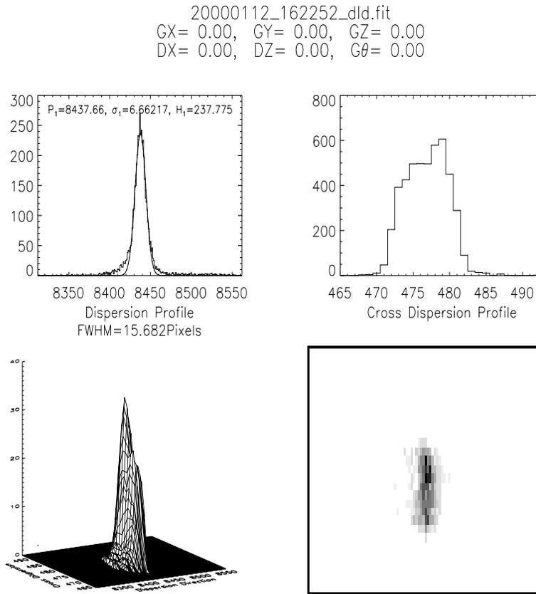
Figure 2: Sample G130M-C image of the Platinum emission line at  $1283.7\text{Å}$ , near the center of the G130M pass band. The pixel size is approximately  $2.4\mu\text{m}$  (dispersion) by  $33\mu\text{m}$  (cross dispersion). The local dispersion is  $1.57\text{Å}/\text{mm}$ .
