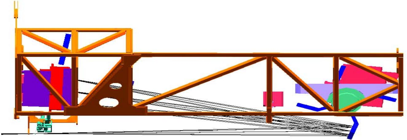
Figure 2: A layout of COS FUV Channel. The light path is represented by the thin lines. Light enters through the aperture at the lower left, and bounces off one of four possible optics on the selection mechanism in the lower right. Light is diffracted and reimaged onto the detector, shown on the left above the input aperture. In one exposure, 300 Å of coverage is provided at 20,000 resolution.
