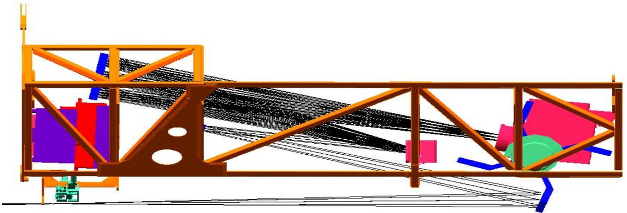
Figure 3: A layout of the COS NUV channel. Light again enters from the same aperture, and is reimaged and corrected by the NUV first optic (lower right). Light is then collimated with a small optic, and reflected to the selected flat, uniform groove density grating which can be tilted to access the desired wavelength range. Three camera optics (upper left) then reimage three stripes onto the MAMA detector (far right).
