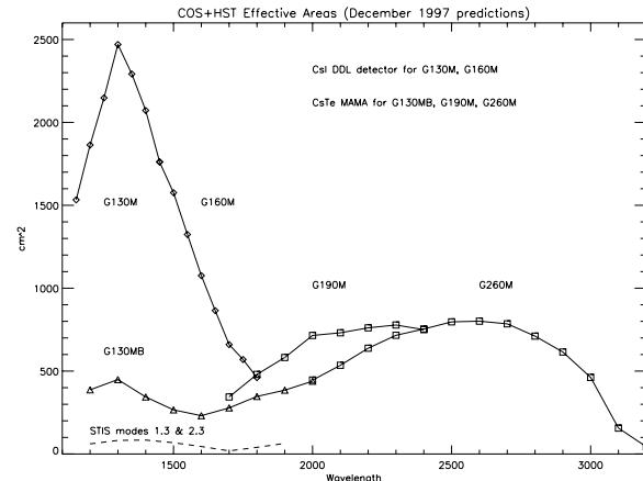
**Figure 2.** Effective area predictions for the COS FUV and NUV high-dispersion grating modes. The effective areas shown include a ‘slit’ transmission of  $\sim 87\%$  through the standard  $2''$  aperture. Effective areas for the STIS echelle modes in the FUV are shown for comparison.
